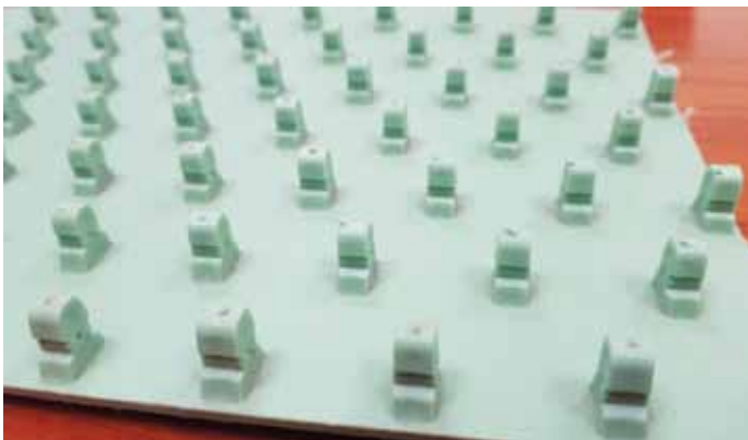
HDPE lining showing anchor knobs
