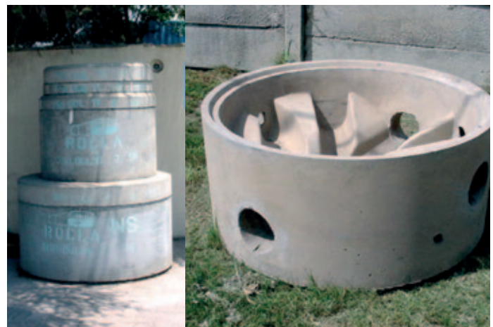
Section of Manhole Access Shaft and Precast Base Unit. 1000 Diameter, Mass 716kg, 6 outlets.
